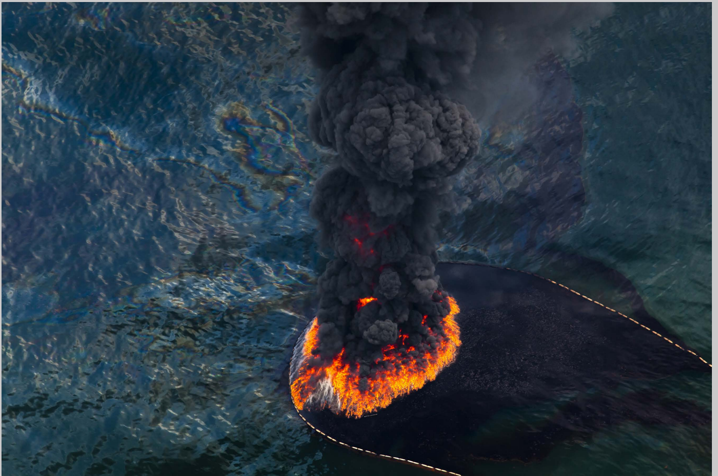
A plume of smoke rises from a burn of collected oil in the Gulf of Mexico. A total of 411 controlled burns were used to try to rid the Gulf of the most visible surface oil leaked from the BP Deep Water Horizon rig in 2010.
